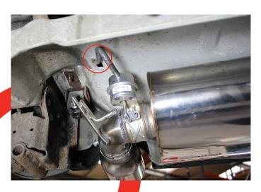
Once the Scorpion system is fitted re-route the vacuum valve hose back on itself, then through the hole in the heat shield as shown in the image, once re-routed connect the hose to the Scorpion valve.
